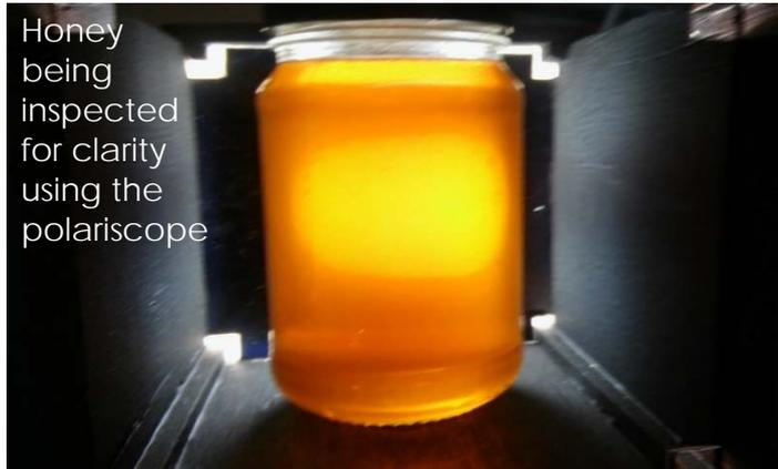
Honey being inspected for clarity using the polariscope
