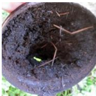
Sooty tar build up
